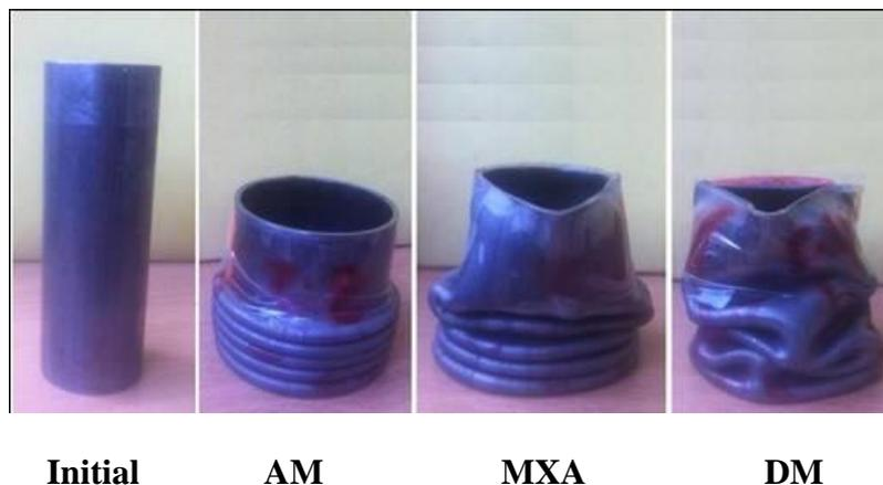
Figure 4. Specimen before and after plastic buckling
