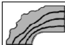
*Figure 4: Section of a laminate around a radius showing the higher  $V_f$  close to the inner radius and the free space left for an easy resin flow close to the outer radius.*
