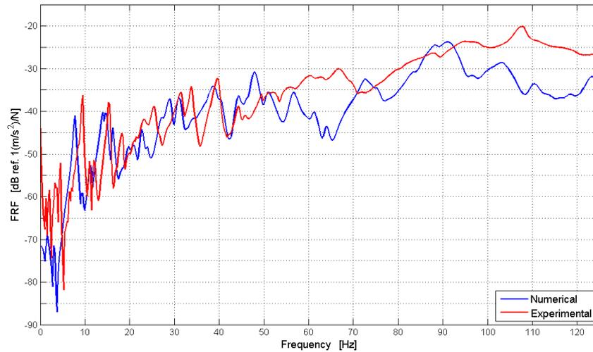
Figure 6: Point FRF's on a selected point of chassis: comparison between experimental and measured curves.
