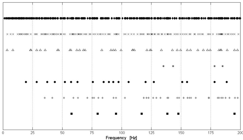
Figure 7: Mode count for components and assemblies.  $\square + \circ *$ : suspended elements in free-free BC,  $\triangle$ : frame in free-free BC  $\times$ : frame assembly in free-free BC,  $\diamond$ : complete vehicle lying on its tires
