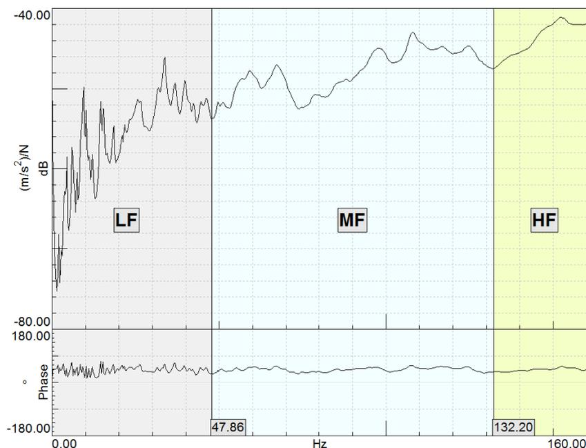
Figure 2: Sum of all the measured FRF's and characteristic frequency ranges.
