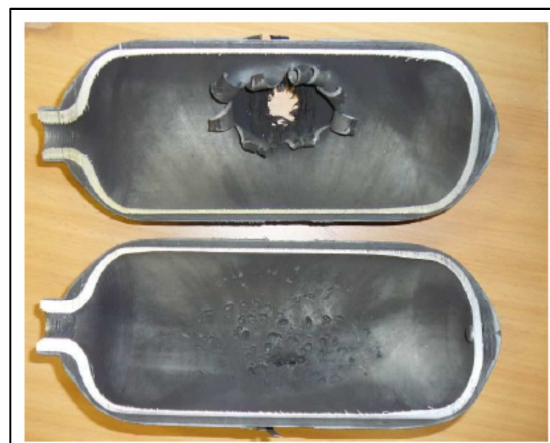
Figure 5. Perforation of tank with large mushrooming for trial with water #HE0208
